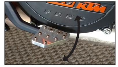
(4) Check brake pedal movement to be sure there is no interference with other parts of your bike. For optimal performance adjust your brake lever height to your preference. Refer to manufacturer's instructions for your specific bike to complete that adjustment.
