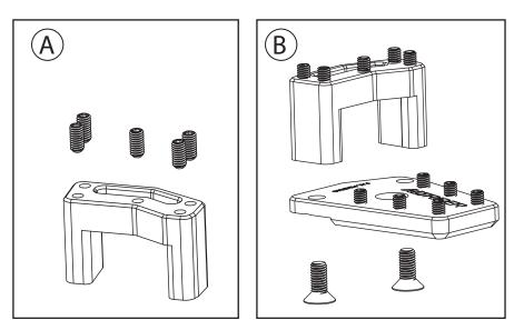
(A) If your kit is equipped with the optional Riser, install the grip pins, with thread locker, in the riser now.
