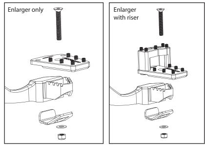
Place enlarger on brake pedal tip. Insert M5 x 35mm screw, and use 8mm socket tool to attach steel lower plate with M5 washer and M5 locknut. Tighten to 4.4Nm.
