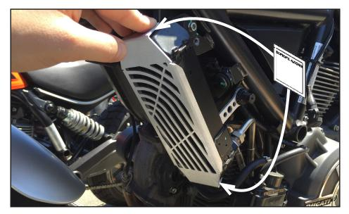
Set the guard aside, using the included isopropyl surface prep pad, clean the top and bottom surfaces of the oil cooler so that no oil, dirt or debris are present. This will ensure the best bond of the high-temp adhesive.
