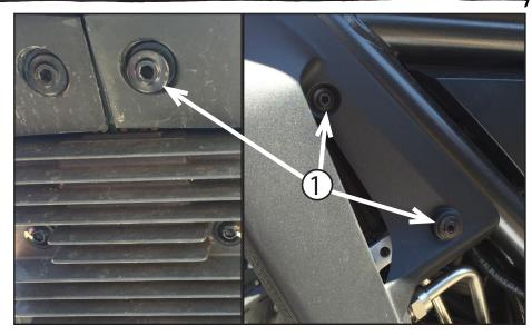
Use a 4mm allen tool to remove the (3) OEM fasteners which hold the plastic oil cooler shroud in place. You will reuse these fasteners.
