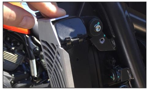
Peel off the backer for both strips of adhesive and carefully place the guard over the cooler. Maintain the 1-2mm gap between the guard and the oil cooler's fins, press down on the top and bottom flanges as shown above to secure the tape to the oil cooler. Put the plastic shroud back on using a 4mm allen tool and your installation is complete!
