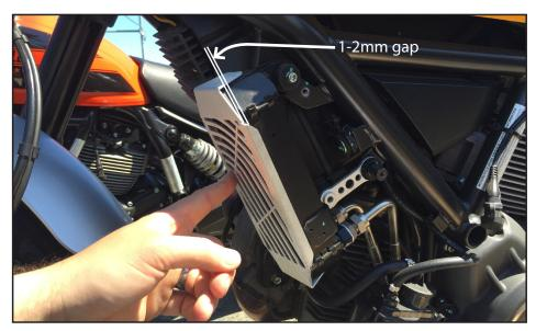
Before peeling the backer off of the high temp VHB adhesive, place the guard over the now exposed oil cooler to get a feel for how it will fit. You will want a small gap of 1-2 mm between the cooler fins and the guard once installed.
