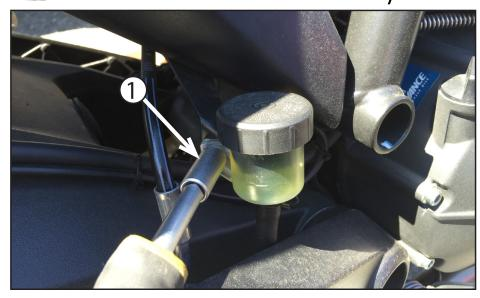
(1) Use an 8mm socket to remove the OEM M6 hex bolt. You will not reuse this bolt.
