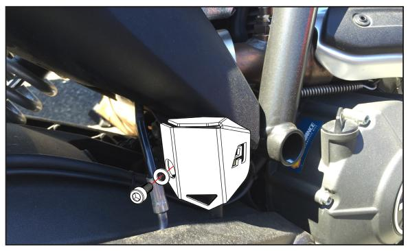
Using a 5mm allen tool, follow the assembly order shown above and attach the reservoir guard as shown. Tighten the provided M6 down (to 4nm) and you are finished.
