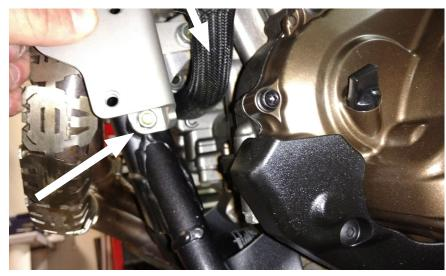
Insert the M8 x 100 socket cap screw and washer through the AltRider bracket and through the engine case. This will be easier to do if the bracket is pulled slightly outward loosely.
