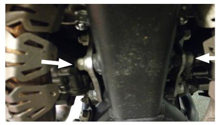
!! TIP If the screw insertion is difficult, use two 12mm spanners to loosen the last M8 bolt and nut, just enough to allow the brackets to move and allow easy screw insertion.
