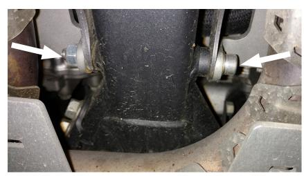
Screw the M8 x100 socket cap screw into the M8 lock nut and washer.
