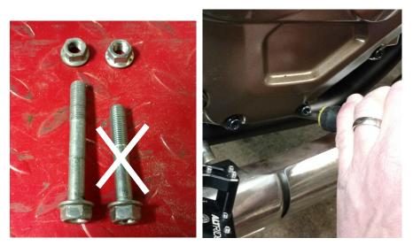
6 Remove both screws. discard the forward, shorter (60mm) screw, but keep the nut. !!TIP If removing the screws is difficult, wrap a screwdriver or small pry bar with cloth and lever the frame rail downward to release the pressure on the screw.
