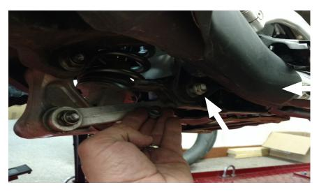
(4) Use 12mm spanner and socket and remove the lower exhaust hanging bolt. The entire loosened system will now hang slightly lower.
