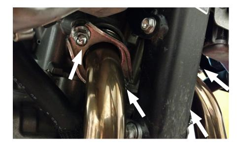
② Use 12mm socket with extension, loosen the four (4) acorn nuts that hold the exhaust header flanges. Do not remove completely, but make very loose.
