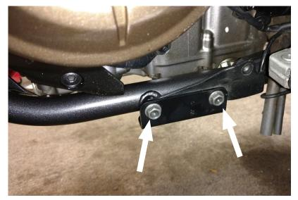
Remove two (2) M8 hex cap screws from the left rear frame rail. (If AltRider skid plate bracket is alread installed, leave it in place).
