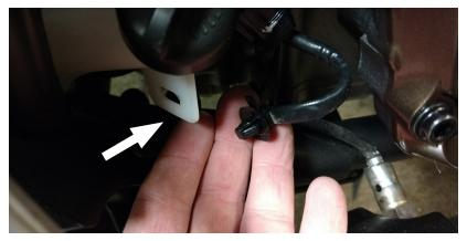
① Depress locking tabs and unfasten the small clip that holds the oxygen sensor wire to the fill reservoir (located near the rear brake pedal).
