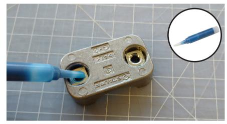
Add medium-strength thread locker to each of the inserted nuts in the four (qty 4) clamp halves.
