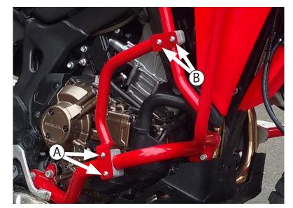
(A) Attach the lower 1.25" clamps, using the M6x50mm long button head screws with washers. Leave loose for now.
