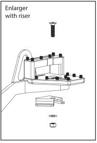
Place enlarger on brake pedal tip. Insert M5 x 35mm screw, and use 8mm socket tool to attach steel lower plate with M5 washer and M5 locknut. Tighten to 4.4Nm.
