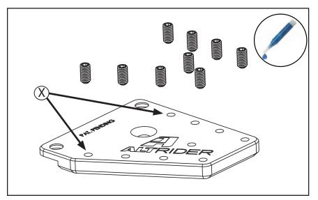
1 Install M4 x 8mm Grip pins, using 2mm Allen driver. Use a small dot of thread locker on each pin. Total number and placement is up to you. Tighten snug, but be careful not to strip the tool. If installing the riser, do not install a pin in positions marked (X)
