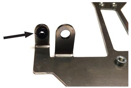
Remove rubber grommet from Honda belly pan and insert into AltRider rear bracket as shown. TIP! A dab of water will help it slide into place easier.
