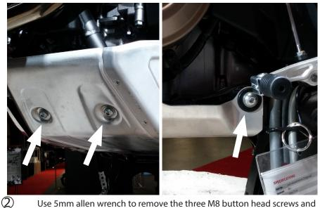
Use 5mm allen wrench to remove the three M8 button head screws and remove OEM belly pan. You will not re-use these screws.
