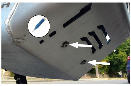
Hold the AltRider skid plate in place and install the front two M8 cap head screws with washers. Apply a drop of thread locker to each screw. Just get the screws started, and leave loose during installation.
