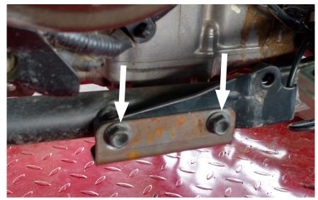
Place the rear bracket over the small OEM hose routing bracket and reinstall the two M8 hex head screws finger tight.
