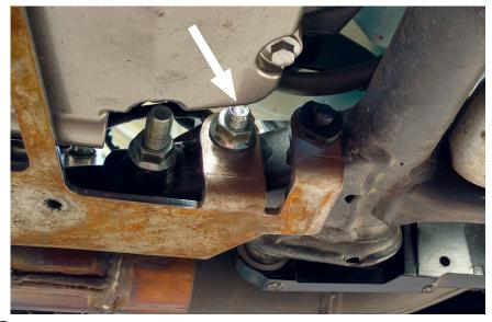
(8) Go back and tighten the M10 frame bolt completely (use two 14mm spanners or spanner + adjustable wrench).
