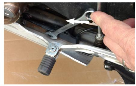
(12) Use 12mm spanner to fully tighten the two hex head bolts on the rear bracket as shown.
