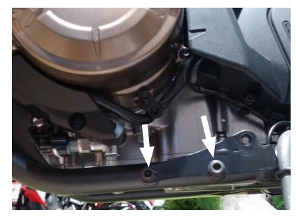
Use 12mm socket and remove the two hex head M8 screws from the small bracket as shown. Save these screws for reinstallation. Leave the OEM hose bracket in place.
