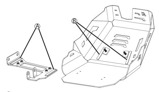
Apply rubber adhesive strips on skid plate and on bracket.
