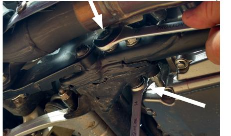
Use two 14mm spanners to loosen the right rear frame bolt. If you have one spanner and one adjustable wrench, use the adjustable wrench to hold the bolt head stationary while using the spanner to loosen the nut. Remove the nut and save for reinstallation.
