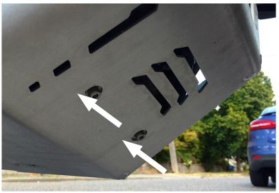
Tighten the two from M8 screws fully to 15 Nm.
