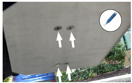
10 Attach skid to rear bracket, use four M8 flathead screws as shown. Apply a drop of loctite to each screw. Get each screw started by hand. Tighten each screw in sequence, working from screw to screw in turn until each is up to 10 Nm.
