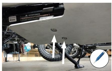
Add a drop of thread locker to each M8 x 20 cap head screw. Raise rear of skid plate into position. Insert screws with washers and torque to 18 Nm
