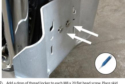
Add a drop of thread locker to each M8 x 20 flat head screw. Place skid plate and insert front M8 x 20 flat head screws very loose.
