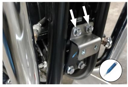
Add a drop of thread locker to each M8 x 20 hex head screw. Use 13mm socket to install upper bracket with two screws with washers. Leave finger tight for now.
