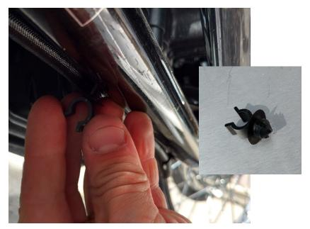
$\mathfrak{Z}$  Remove plastic cable clip from right side frame rail, near oil filter.
