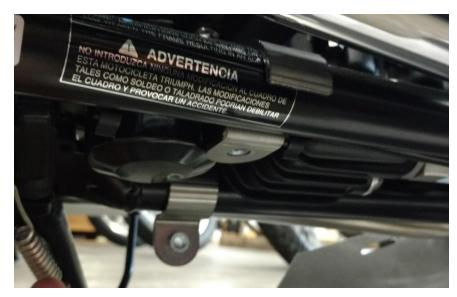
Place rear brackets around frame rails as shown, with mounting hole toward center of bike. Be sure wires are situated above bracket.
