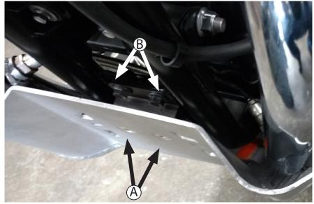
(A) Tighten front M8 flathead screws to 15 Nm.(B) Use 13mm spanner to tighten hex cap screws to 18 Nm.
