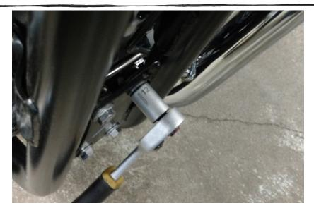
Use 12mm socket and remove the upper two bolts on the front frame plate.
