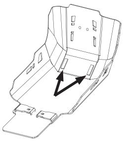
(5) Install rubber adhesive strips as shown. 6mm (1/4") from edge, centered lengthwise.
