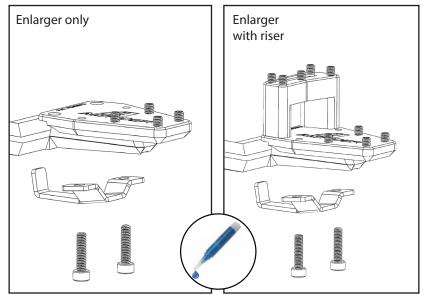
Place enlarger on brake pedal tip. Add a drop of thread locker to each M4 x 16mm cap head screw. Insert the screws from below, through the steel plate. , tighten to 5Nm.
