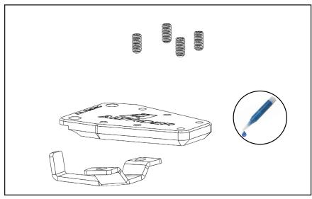
Install M4 x 8mm Grip pins, using 2mm Allen driver. Use a small dot of thread locker on each pin. Tighten snug, but be careful not to strip the tool.
