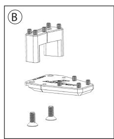
(A) If your kit is equipped with the optional Riser, install the grip pins with thread locker in the riser now.(B)Then apply drop of thread locker to the two M5 x 12mm flat head screws, and attach to the enlarger base.
