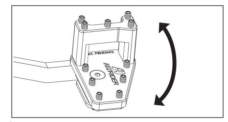
(4) Check brake pedal movement to be sure there is no interference with other parts of your bike. If the riser is installed, adjust your brake pedal height so that in the seated position you are using the enlarger, while in the standing position you will use the riser. Adjust your pedal height using the manufacturer's instructions to ensure correct procedure. It is important to set the correct free play to avoid caliper drag and potential brake failure.
