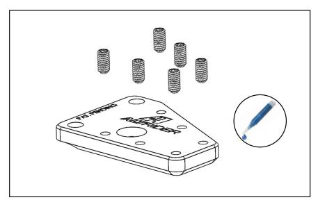
Install M4 x 8mm Grip pins, using 2mm Allen driver. Use a small dot of thread locker on each pin. Total number and placement is up to you. Tighten snug, but be careful not to strip the tool.
