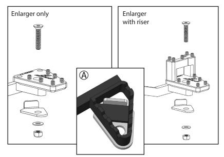
(A) Steel lower plate should be aligned as shown.
