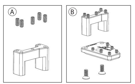
(A) If your kit is equipped with the optional Riser, install the grip pins with thread locker in the riser now.
