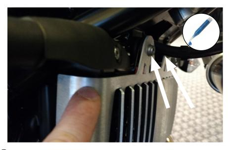
③ Replace M6 OEM screws, use a drop of loctite on each screw. Torque to 7Nm
