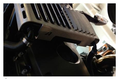
② Fit AltRider oil cooler guard in place. Slid up from below, make sure that the rubber bumpers are placed correctly and do not become dislodged.
