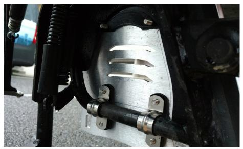
Place the skid plate in position, with the threaded studs passing through the tube spacers and U-clamps.
