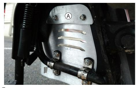
(A) Sandwich the front mount with the second flat spacer, then the aluminum front bracket.
