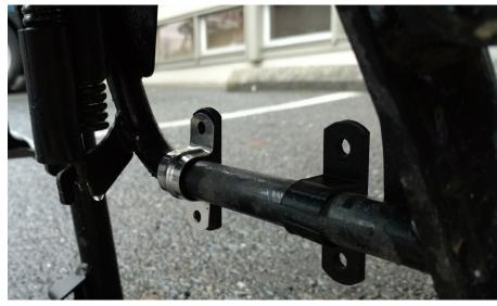
Place motorcycle on the center stand. Snap plastic tube spacers on to the center stand cross tube as shown. Place U-clamps over spacers.
