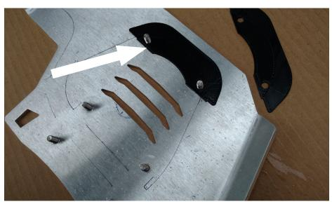
Place one of the flat spacers onto the forward two threaded stud. Be sure that the smooth side is placed against the AltRider skid plate.
