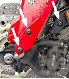
(A) Attach the Right and left large lower brackets. Add a drop of loctite to each screw. Insert the flat head screw in the upper position and the button head screw with washer in the lower position. Be sure on the left side to route the ABS wire under the bracket, between the mounting bosses.
