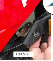
3 Attach the Right and Left small upper brackets. Add a drop of loctite to each screw. Insert the flat head screw and screw tight to 6 Nm. Note location of anti-rotation tab, be sure it is snug against the top edge of the mounting arm. This tab prevents the rear edge of the fender from moving closer to the tire tread. If needed, use pliers to hold it in place as you tighten the screw.
