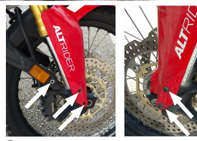
Use 5mm hex allen tool and remove six (qty 6) OEM fasteners from the front fender. Remove and save the shoulder washers. Save all for reinstallation.
