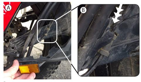
(A) Unclip the left side cover. Note how it goes together for reinstallation. (B) Move the ABS sensor wire (if equipped) as shown, by inserting the rubber grommet in a slightly lower position in it's plastic clip. This gives additional length to the wire needed. Clip the cover back in place.
