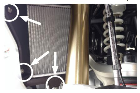
Using a T25 driver, remove the (3) oem screws holding the shroud over the radiator on each side (6 total screws). Save these for reinstallation.
