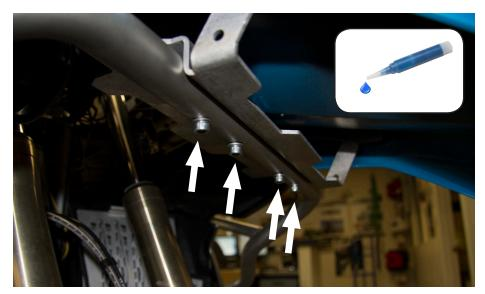
Hold your upper bars in place while you start threading the (4) M6 x 35 mm fasteners and washers. Add thread locker to each fastener, do not tighten all the way. (Bracket may differ slightly from picture depending on model).
