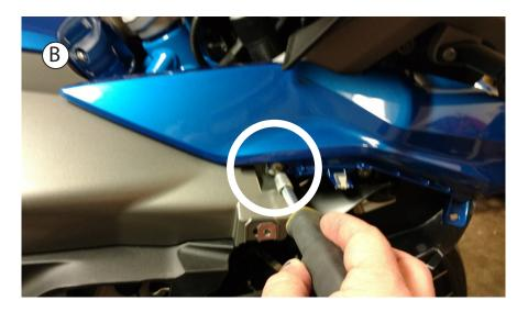
3 Remove the four (4) screws (two each side) at the rear of the beak plastic. (A) One on top near the tank, (B) one on the side just under the edge. (Left side of bike only shown in the pics above)
