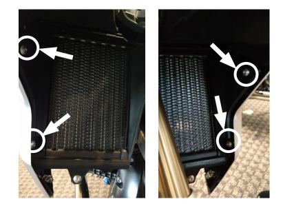
Using T25 driver remove the (4) screws holding radiator shrouds in place, (2) on each side.
