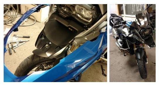
(5) Gently pull the beak forward to remove it. Note rubber grommets and other mounting points for reinstallation.
