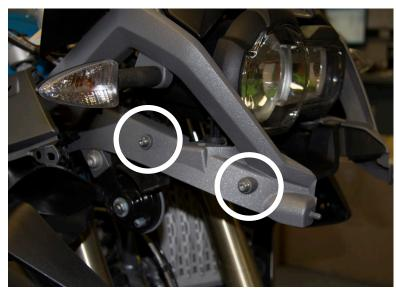
6 Remove (4) total OEM M5 screws from the front sub frame (2) on each side. Set them aside as you will not need them to complete this installation.
