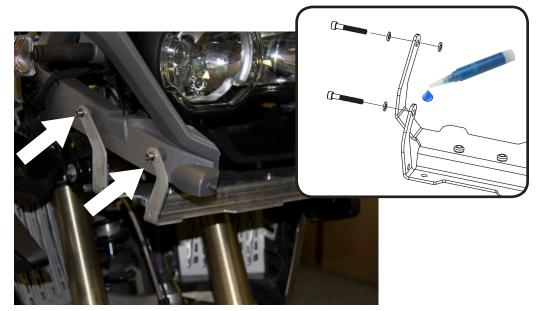
Install the upper bracket using an M4 driver and (4) M5 x 35mm bolts and (6) M5 washers; TAKE NOTE OF WASHER PLACEMENT BY REFERENCING THE ABOVE DIAGRAM. Apply thread locker to the fasteners. Completely tighten each fastener and torque to 10 nm.
