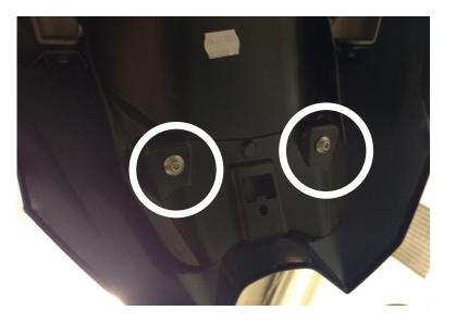
(4) Remove the two (2) fasteners just under the front edge of the beak.
