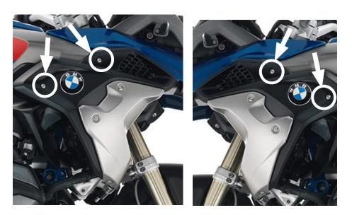
① Using T25 driver, remove four (4) screws holding the side panels in place, (two fasteners on each side) where indicated. Note: pay close attention to where each fastener comes from, some are different lengths.
