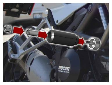
A Now assemble the second side of the frame sliders as shown. Using (2) 18mm sockets w/extensions, tighten both sides down. Use the torque wrench to tighten both sides to 60Nm.
