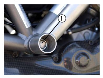
Using (2) 18mm sockets w/ratchets, remove the AltRider provided through bolt from the Crash Bars' frame mount.
