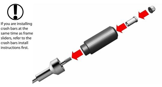
Assemble one side of the sliders as shown above. Tighten the M12 locking nut with an 18mm socket so that just one thread is showing past the top of the nut. Do not tighten all the way just yet.
