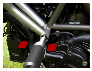
3 Insert the assembly through the crash bars' frame mount as shown above. Push this whole assembly through until the frame slider is seated firmly in the crash bars.
