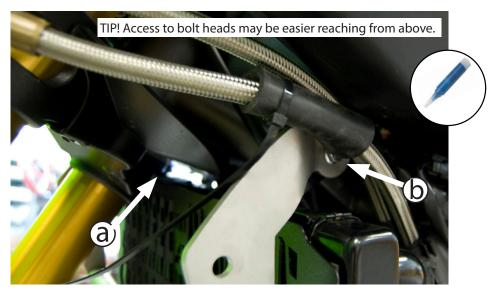
(Shown with fairings removed for clarity) Using a 10mm socket and driver, remove the left side upper radiator mount bolt. Attach the bracket in place as shown and use (1) M6 x25 fastener with loctite to mount the bracket (note bracket bends away from bike centerline toward edge of radiator). Install right side bracket in same manner. Leave bolts finger tight. TIP: unclip the oil cooler line.
