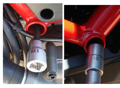
Using an 8mm allen key on one side and a 15mm socket on the other, remove the motor mount through bolt.
