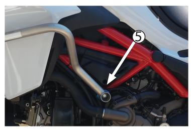
Insert one M12 washer into the frame socket.
