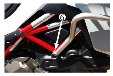
6 Insert one M12 washer into the frame socket.
