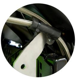
Take the rubber tube provided and use scissors to split it. Wrap it around the stainless oil line and zip-tie it in place as shown above.
