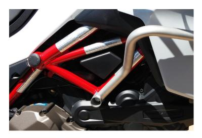
(1) Use both 18mm sockets to tightern both engine bolt lock nuts to 60Nm.
