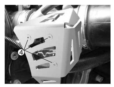
Use a 2.5 allen wrench to fasten the 3 remaining screws. Do not over-tighten!
