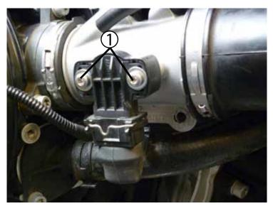
Use a t20 torx wrench to remove the OEM hardware (including the washers). Store these in a safe place.
