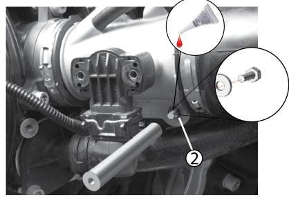
Put one drop of loctite (provided) on the last couple of threads of the M4 fastener. Use a 8mm spanner to tighten the spacer, and a 7mm spanner to hold the hex screw. Do not over tighten!
