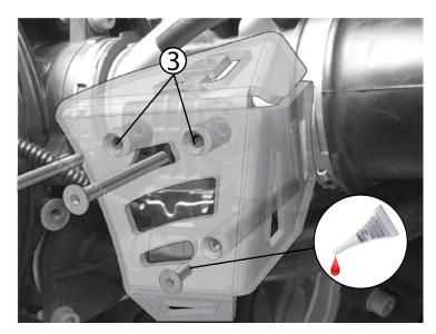
Apply loctite to the last couple of threads of the M4x12 flat head. Using the long M4 flat heads to hold the spacers in place, put your new potentiometer guard on the potentiometer.
