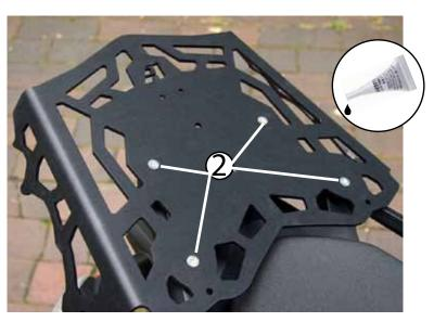
Line up the luggage rack mount holes. Using a 4mm allen tool, insert the (4) M6 flat head fasteners. Do not forget to apply thread locker! One drop at the end of each fastener is plenty.
