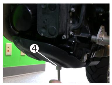
Using a 13mm socket, remove all four of the nuts holding the OEM skid plate in place. Remove the skid plate.
