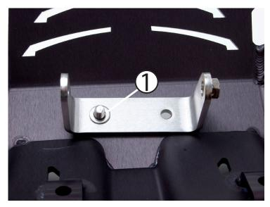
Insert the M8 flat head fasteners in to the holes on the front of the Skid Plate. Place the stainless bracket as shown, and put the washer over each fastener. (the welded nut on the right)
