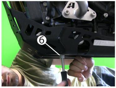
Hold the Skid Plate in place while using a 13mm socket to get the first couple of nuts started. Just a few turns here, do not tighten these all the way down yet.
