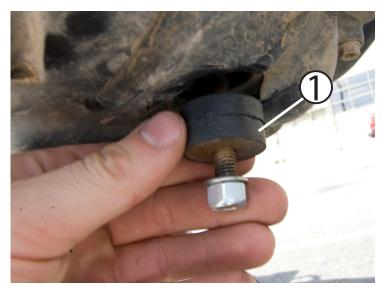
Using your hands, insert the (4) vibration isolation mounts in the mounting holes on the sump of your motor. Finger tighten all (4) for now.
