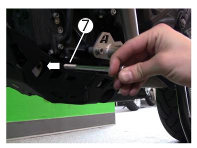
Using a 13mm socket w/extension, put the AltRider provided through-bolt in place as shown. Just thread the bolt into the weld-nut on the stainless steel bracket. Tighten this down!
