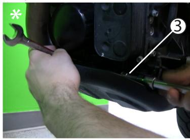
3 \*(pre-2011 F800 models only) Using a T-45 bit with an extension, and a 13mm wrench, remove the front through-bolt on the OEM skid plate.
