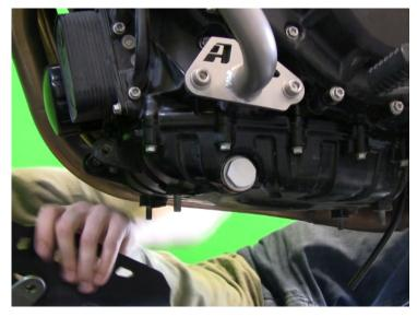
Put the skid plate into position, line up the rear holes first, then the front ones, finally ensuring the front mount bracket slides into place properly.
