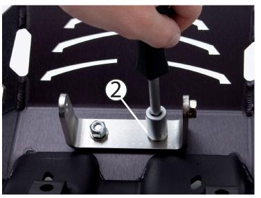
Using a 13mm socket or wrench, tighten the locking nuts on to the exposed ends of the M8s.
