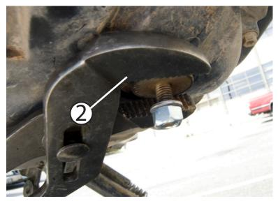
Using a pair of channel locks, gently tighten the vibration isolation mounts the rest of the way. You will only need aroun 1/8 of a turn just to seat the vibration isolation mounts agianst the sump. Do not overtighten! If you are twisting the rubber m, the mounts are tight. F650GS specific hardware installation steps complete. Move on to next page and begin at step 1 to begin the skid plate installation. You will skid steps 3 and 4.
