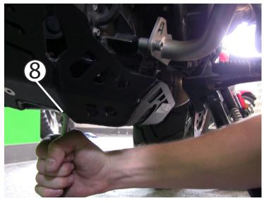
Using a 13mm socket, tighten all of the vibration isolation mount nuts down. After 100 miles check all fasteners to ensure they are tightened correctly.
