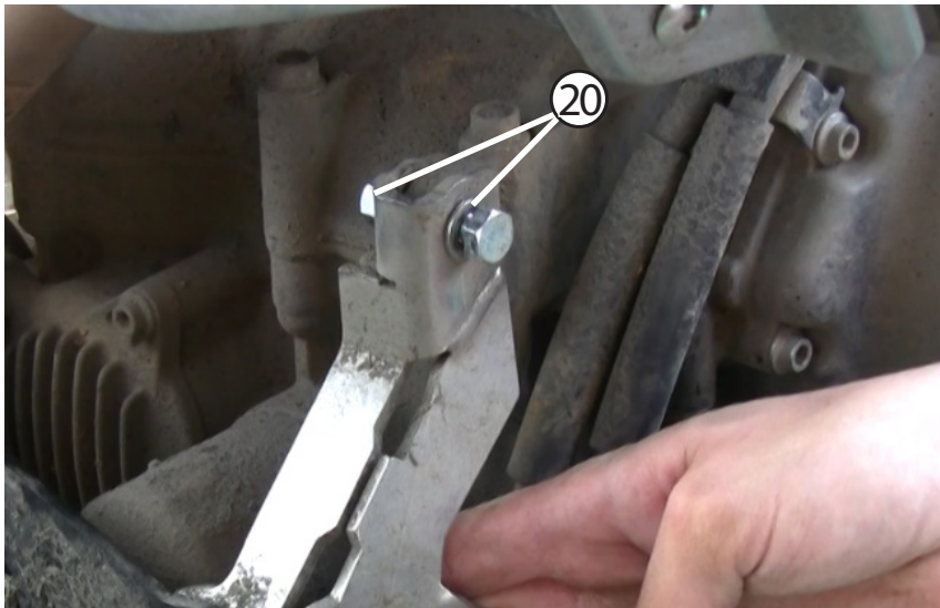
19 Last, you will tighten this bolt using a 13mm socket and 13mm wrench. Tighten to 10 Nm.
