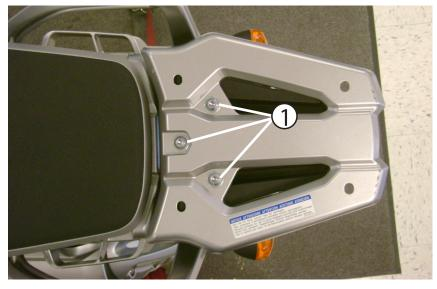
Using a 6mm allen tool, remove the 3 fasteners indicated, and remove the OEM silver luggage rack, then using a 6mm allen tool, remove the black plastic OEM luggage rack support.
