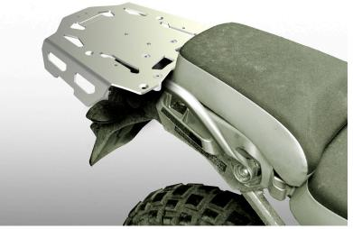
The AltRider luggage rack can also be configured as shown. You'll need to remove the grab handles to use the rack in this configuration. This configuration puts the rack level with the cargo platform under the pillion seat.
