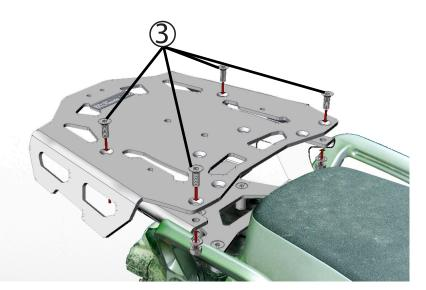
Using a 13mm spanner and a 5mm allen tool, assemble the top rack onto the mount bracket as shown. The assembly order should go: M8 nut - M8 washer - mount bracket - top rack - M8 flat head fasteners.
