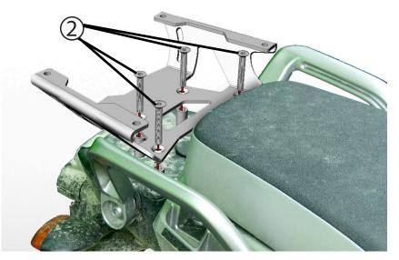
Using a 5mm allen tool, assemble the luggage rack onto the tail of the bike as shown. The order of assembly should go: mount points - provided spacers - mounting bracket - M8 fasteners. Note that the two longer standoffs go closest to the seat.
