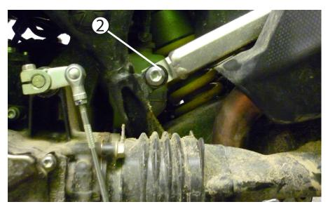
Using a 14mm wrench and t50 torx tool, remove the nut on the back of this fastener. Leave the OEM fastener in place, just pull the nut off of the back.
