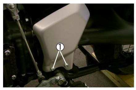
(1) Remove these (2) OEM fasteners.
