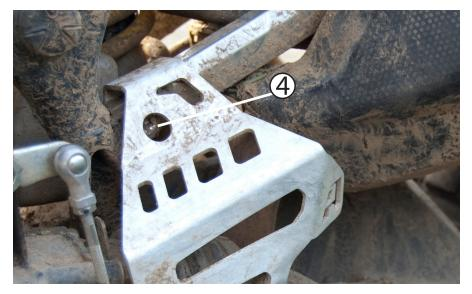
After applying a drop of thread locker to the inside of the OEM nut, use the 14mm wrench and t50 torx tool to tighten it down.
