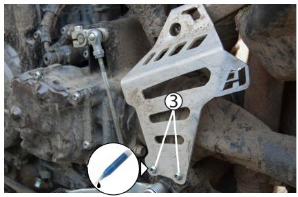
Install the AltRider Universal Joint Guard. After applying thread locker to the last couple of threads on the (2) OEM fasteners, use a 4mm allen tool to tighten these down. Make sure the tab on the top is lined up with the OEM bolt.
