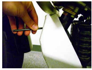
Use one hand (or a knee) to stabilize the skid plate while inserting the M6 with a right-angle hex wrench. The cut outs were designed specifically to allow for this. Tighten 4 turns.
