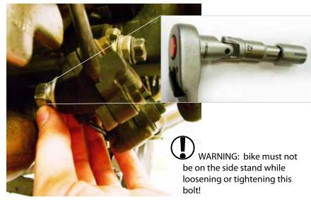
Use a 17mm spanner or the inset Proxxon assembly to remove the bolt on the inside of the side stand mounting bracket.
