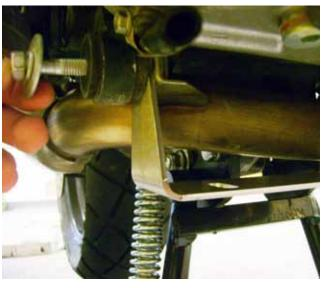
Note: the mounting bracket is not symmetrical. The small hole should go on the side with the exhaust hanger. Also the slanted portion edges should always face the front of the bike.
