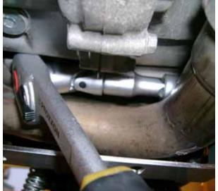
If you have the 56pc Proxxon toolset we recommend using the configuration shown to tighten the side stand hanger bolt.
