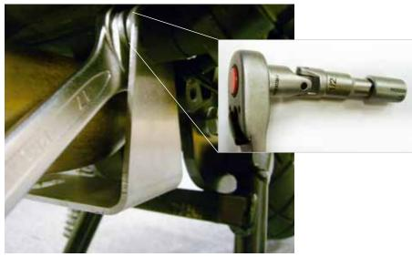
Use a 17mm spanner or the inset Proxxon assembly to tighten the bolt just enough to make the bracket stiff, but moveable.
