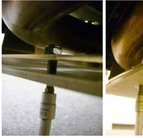
With the skid plate loosely bolted up front, you can move to the back and place the M8/washer/nut assembly with the washer/nut on top of the bracket. You'll need a 13mm wrench for the nut.
