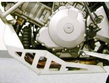
Your assembly should look like this. Now you can go back and tighten all the bolts: (a) Tighten M8 bracket bolts. Make sure bracket is flat on the skid plate. (b) Tighten 4 M6s up front.
