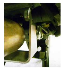
Slide the skid plate bracket in between the exhaust hanger and the exhaust flange. Reinsert the bolt/washer and finger tighten.
