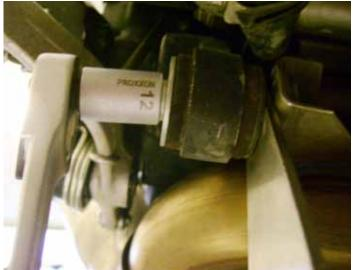
Use a 12mm spanner or a socket to tighten the bolt on the exhaust hanger, tension as step 7.
