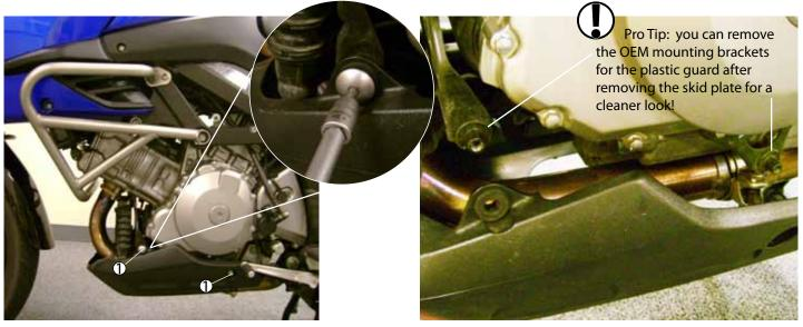
Remove the four button head fasteners from the existing belly pan. There are two on the left and two on the right side.
