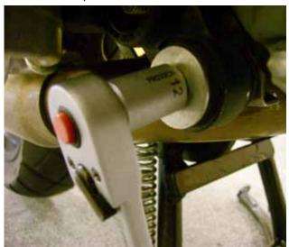
Use a 12mm spanner or a socket to remove the bolt from the exhaust hanger on the right side.
