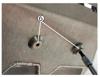
6 Come back to the front and use a 5mm allen tool to tighten these (2) front fasteners down.
