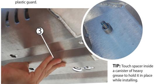
Insert the (2) M8 x 35 flat head fasteners, (2) finishing washers and (2) spacers in that order. The spacers should be on the inside of the skid plate, and the finishing washers on the outside. Apply thread locker to the M8 fasteners then get the Skid Plate in position.
