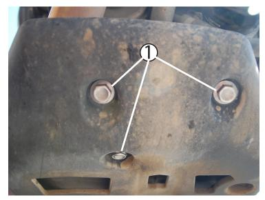
Using a 12mm socket and ratchet, remove the (2) OEM flanged hex cap fasteners in the very front, then remove the (2) OEM nuts toward the front on the bottom of the
