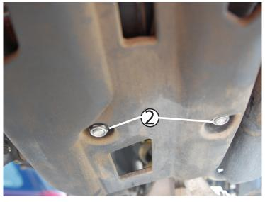
Using a 12mm socket and ratchet, remove the (2) OEM nuts in the rear of the guard and remove it.
