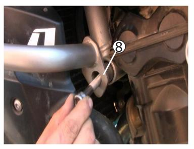
Reinstall the OEM M10 engine bolt without washer but do not tighten completely.
