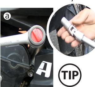
Remove the 2 upper M10 engine bolts using an extension, universal joint and M14 socket reach behind the frame (a) then use an M8 allen key (or T50 Torx, 2014 and on) (b) to hold and remove. Be careful to capture nut when it comes loose. You will re-use the left side bolt but not the right side bolt.
