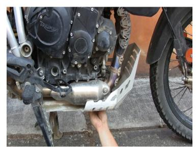
If OEM or aftermarkert skid plate is installed remove this now.
