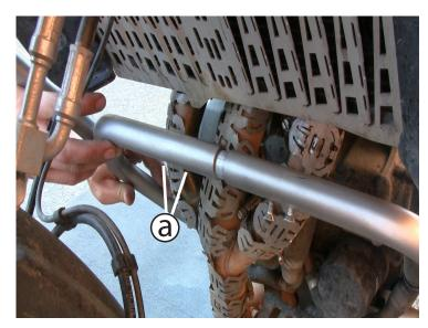
Install right side crash bar by sliding over center connector and lining bar up with both upper and lower mounts. (a) Start the (2) remaining M6 x 20 flat head screws into center connector.
