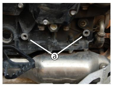
Remove (3) black plugs. (2) on right side [a] as shown and (1) on left side. Right side plugs have already been removed in example photo.
