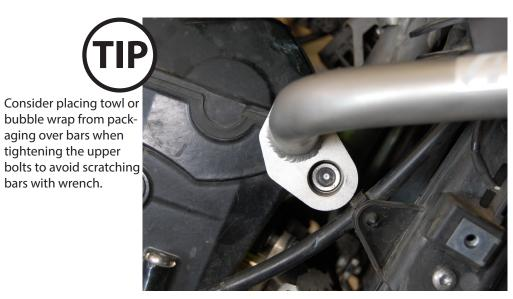
Install the AltRider provided M10 x 70mm socket head cap bolt but do not tighten all the way.
