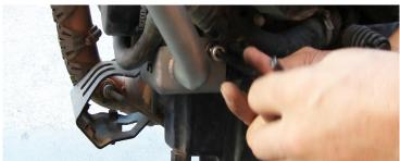
Install left bar by sliding the lower flange in front of coolant hose. Start the OEM Hex (socket cap shown) bolts but do not tighten completely.
