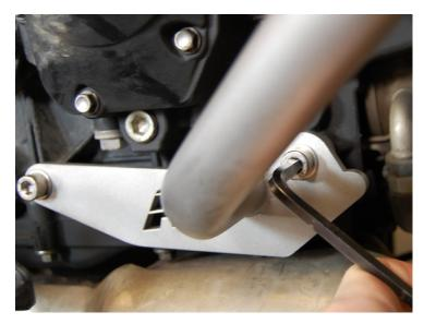
Tighten all (4) lower mount bolts to 20nm of torque. There are (2) bolts on each side.
