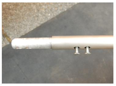
Take the 6.75" aluminum connector and the left side crash bar. Start (2) of the M6 flat head screws but do not fully tighten. You will tighten these later in the installation.
