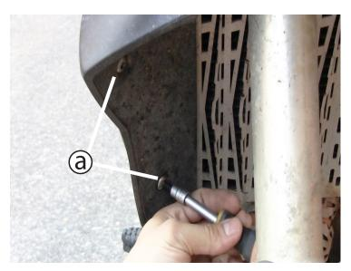
Remove the right side radiator shroud using an M5 allen. There are (3) screws to remove. (1) screw is on the outside and (2) are on the inside [a].
