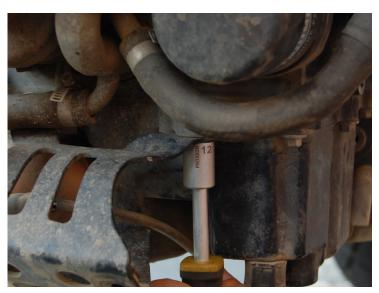
Remove 12mm Hex bolt on on left side directly underneath the oil filter. Save this bolt but you will need it later in the installation.
