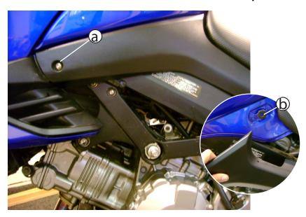
(a) Using a 4mm allen, remove the fastener on both sides of the bike. (b) After the fastener is removed it's held on only by rubber grommets, remove the plastic covers.
