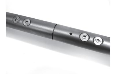
(a) Using a 5mm allen, insert the two M8 button head screws (with M8 washers) into the top mount flange. Torque the M8s to 20Nm (b) Replace the through-bolt nut and tighten until the locking nut engages the bolt.
