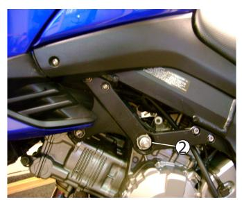
Now set a 17mm socket in place on the motor mount nut. You will turn this side while holding the right side.
