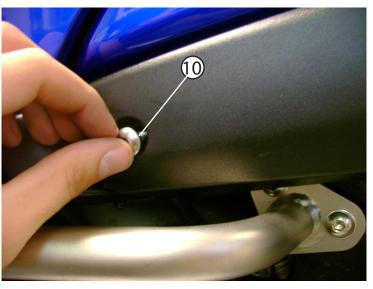
(10) Replace the plastic cover pieces on both sides and reinsert the OEM fasteners. Do not over-tighten!
