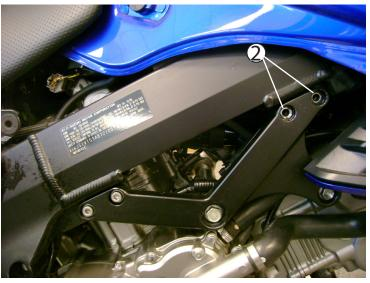
Using a 6mm allen, remove the two top casting bolts on the right side where indicated.
