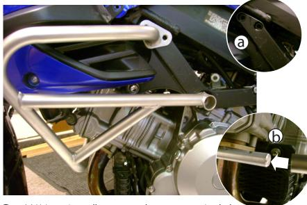
(a) Using a 6mm allen, remove the two top casting bolts.
