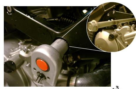
$\bigcirc$  Remove the through-bolt as indicated above.
