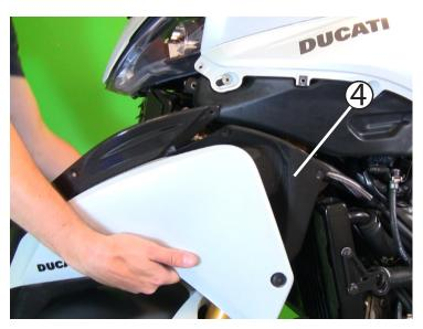
Very carefully remove the fairing/beak. Watch for the 'floating' panels to get caught on things. Take your time and do this carefully, especially on the S model w/carbon fiber.
