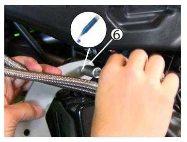
(6) Using a 10mm socket and driver, remove the left side radiator mount bolt. Now put the crash bar bracket in place as shown and use (2) M6 x25 fasteners to mount the bracket (bends away from bike centerline). Do this on both sides and leave it just loose enough to move the bracket. TIP: unclip the oil cooler line.
