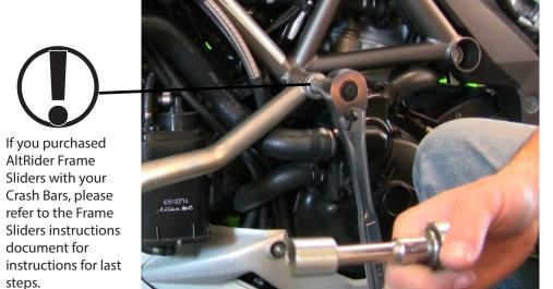
Now using both of your 18mm sockets w/extensions, tighten the (2) lock nuts all the way down to 60 Nm.
