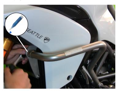
Using a 15mm socket, tighten the hex cap fasteners into the crash bars on both sides. turning the front wheel can give you better access for this step. **Don't forget thread locker!**
