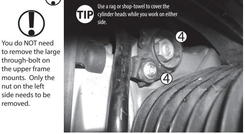
Now you'll need two 18mm sockets. Your helper can hold the bolt on the riders right side while you turn the nut on the left side of the bike. Remove this nut completely. Also remove the T30 torx fastener.
