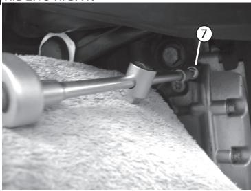
6 Now remove the T30 torx screw on the riders right side, upper frame mount. On 2010 and newer models this screw is not present. AltRider provides a replacement both for the left and right sides. See kit contents #7, #9 and #10.
