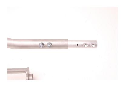
Insert the billet aluminum connector rod in the left side crash bar, start the two M6 flat head screws using a 4mm allen. Leave loose to make starting second set later on much easier.
