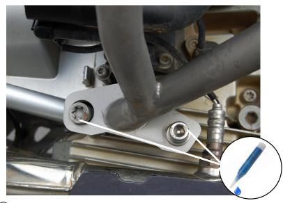
Install the OEM T55 torx with washer and M10 x 60 bolt to left lower mount and OEM T55 torx with washer and M10 x 70 bolt to lower right mount. Do not tourqe all the way down yet. NOTE: the longer M10 x 70 mm bolt belongs on the right side.
