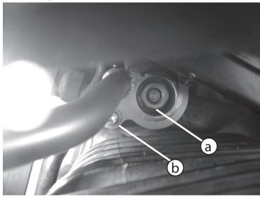
Torque the T30 screw on left side (b) to 8nm and torque the 18mm cross bolt (a) and nut to 82nm.
