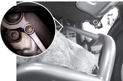
Install right side crash bar. Start by inserting bar on to the connecting rod then line up top and bottom mounts and gently push into place. Use a 4mm allen to insert the (2) remaining M6 flat head screws into the two holes on the underside of the cross-bar. Next using the 10mm wrench install the 6mm hex head bolt and washer into the upper right mount.
