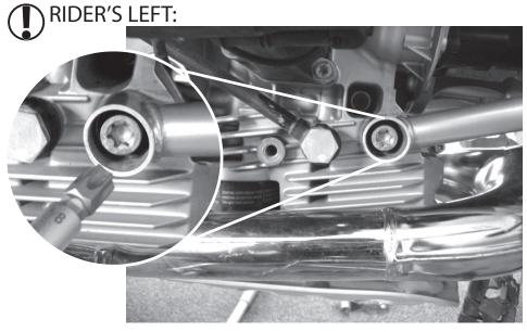
Remove the T55 torx from the lower frame mount on both sides. Be certain you pull the washer out with the fastener.
