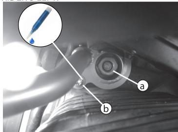
With the aluminum connector installed take the left side crash bar and line up the top and bottom mounts and gently push into place. (a) Install the 18mm nut and leave loose. (b) Install the T30 torx with thread locker, leave loose.
