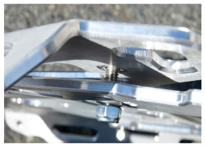
Using a 10mm wrench and a 4mm allen tool, attach the (2) provided brackets to the luggage rack with (4) M6 x 18, (4) M6 washers and (4) M6 locking nuts.
