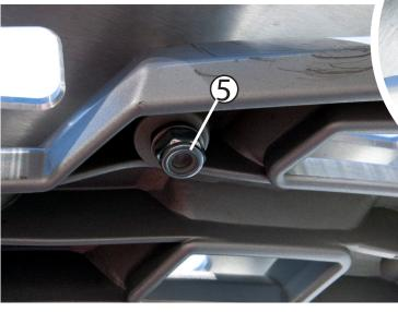
You may need to rotate your spacers to ensure the luggage rack sits flat. Rotate the spacers while the hardware is loose until there are no gaps.
