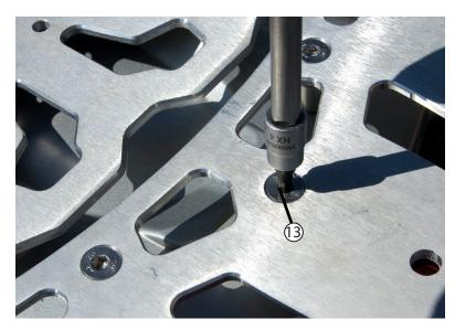
Tighten down the (3) M6 x 40 fasteners using a 4mm allen tool.
