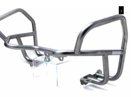
01 Made of 1" stainless steel these stout bars feature ideal mounting points for the ultimate protection. Even with the bars installed you can access the air filter and glove box. 02 A fully kitted out Tenere is ready for the great escape with the AltRider luggage rack and protection. 03 Hand-TIG welds show that no detail is forgotten on the AltRider skid plate. 04 With the AltRider universal joint guard you won't get your pant leg stuck (unlike the OEM set up).
