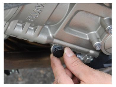
6 Carefully remove the black plastic plugs from the engine case on each side of the bike. The best way to remove these is by spinning counterclockwise like a bolt. If plugs are tight you can use needlenose pliers to start.
