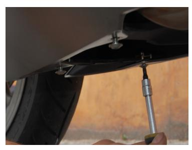
3 Remove the (4) bottom radiator cowl bolts using a T25 driver. There are (2) on each cowl.
