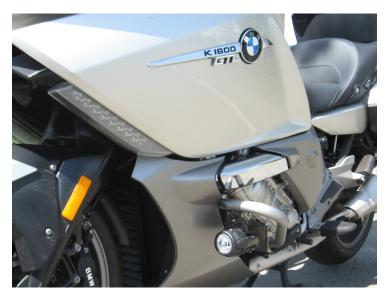
(14) Reinstall both the right and left radiator cowls. Take your time and properly allign the location pin with rubber grommet. Each side requires the (4) OEM T25 bolts.
