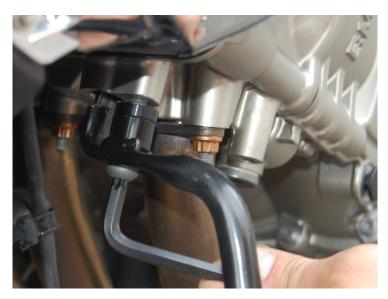
(5) On GTL Model, remove the two Auxillary light brackets using a T40 driver. Be sure to save the bolts and spacers.
