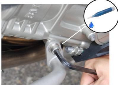
(1) Now that all 4 fastners are started, you can go back around and tighten and tourque fastners to correct spec. M8 x 20 = 19nm and M10 x 35 = 38nm or torque.
