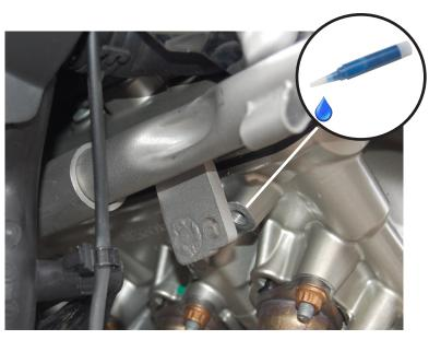
Slide the left side engine bar into the right side and swing the left bar up into position aligning the machined boss + bolt hole on engine case with engine bar mount. Start the M8 Allen bolt w/ washer and threadlocker. Start the M10 Allen bolt w/ washer on lower mount, use threadlocker.
