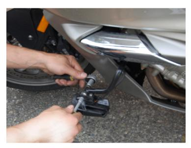
On the GTL Model, first remove the Auxillary lights using a T30 driver and 10mm socket. Next clip the zip ties holding the power cord in place using wire cutters.
