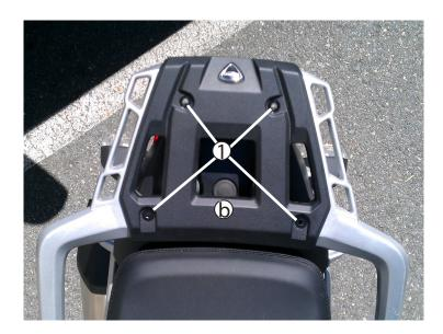
Remove (4) OEM M6 screws and nuts using M4 allen driver and 10mm socket or wrench. Set nuts aside for reinstallation, you will no longer need the screws. Remove plastic cover (a). You will no longer need the black plastic cover.
