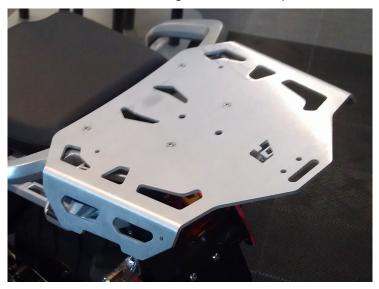
Place AltRider luggage rack on top of spacers and line up holes. Insert the (4) provided M6 x 30mm flat head screws and OEM nuts. Begin to tighten alternating from one screw to another. Torque each screw to 10nm.
